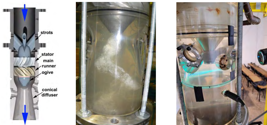
Figure 53. The swirl generator with the main components and the convergent-divergent test section (left). The visualization of the vortex rope obtained in the divergent part of the test section (middle). The visualization of the flow in the divergent part (draft tube cone) when the free runner is installed in the extension of the swirl generator.
