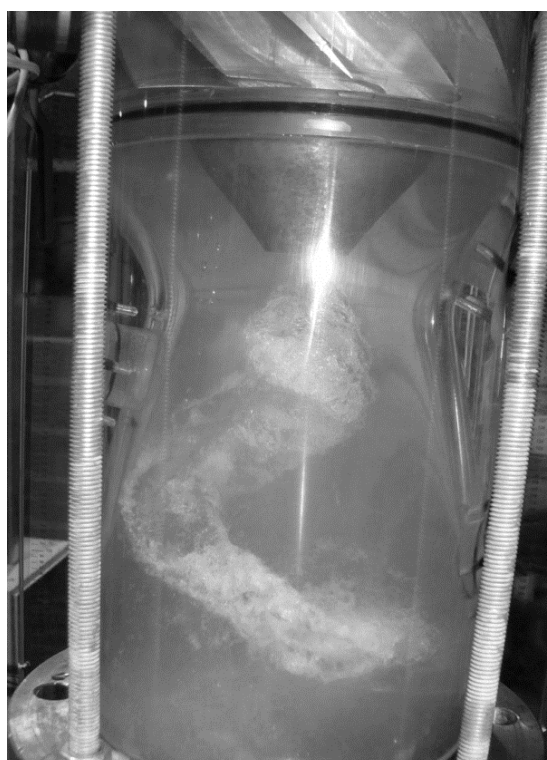
Figure 20. Schematic view of the swirl apparatus and test section from the experimental test rig (left) and visualisation of the cavitating vortex rope in the discharge cone of the test section (right), [29].
