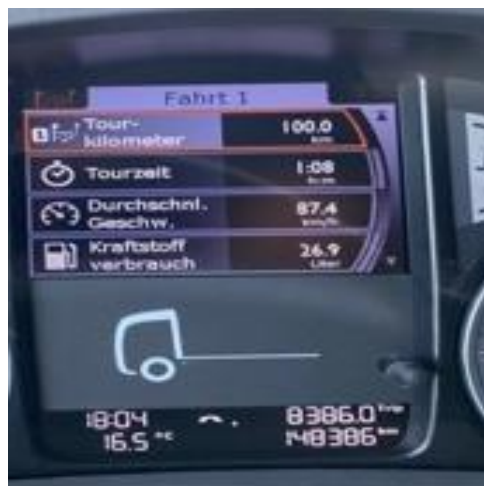
Photo 1: Results recorded on board of the tractor unit Itinerary 1 (Tour kilometer = distance traveled, Tourzeit= travel time, Durchschnittsgeschwindigkeit = average speed, Kraftstoffverbrauch = Fuel consumption) Photo 2: Results recorded on board of the tractor unit Itinerary 2 (Tour kilometer = distance traveled, Tourzeit= travel time, Durchschnittsgeschwindigkeit = average speed, Kraftstoffverbrauch = Fuel consumption)
