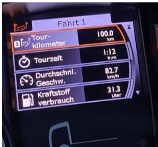
Photo 1: Results recorded on board of the tractor unit Itinerary 1 (Tour kilometer = distance traveled, Tourzeit= travel time, Durchschnittsgeschwindigkeit = average speed, Kraftstoffverbrauch = Fuel consumption) Photo 2: Results recorded on board of the tractor unit Itinerary 2 (Tour kilometer = distance traveled, Tourzeit= travel time, Durchschnittsgeschwindigkeit = average speed, Kraftstoffverbrauch = Fuel consumption)
