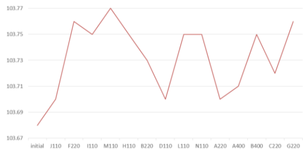
Fig. 5.1.3. Average voltage value at the power system buses for all analyses performed
