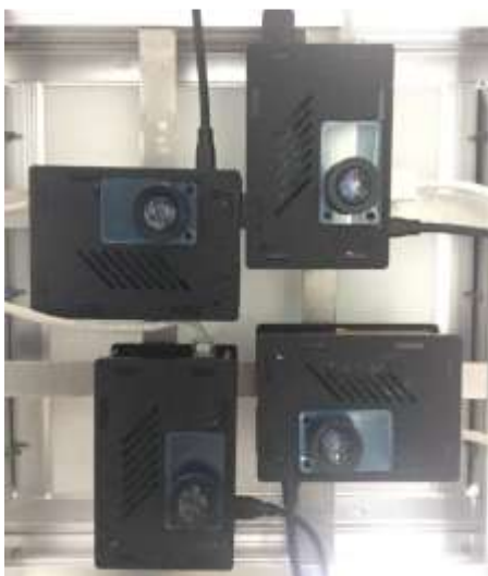
Fig. 4.6-2 The experimental model hardware of the IP-LC-FD. a) The disposal of the four Raspberry Pi - Pi camera ensembles. b) The final experimental model.
