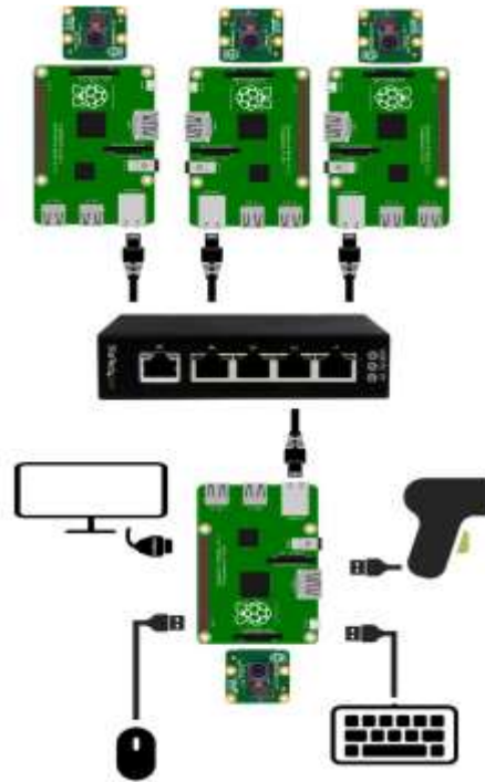
Fig. 4.6-1 The hardware architecture of the IP-LC-FD experimental model.
