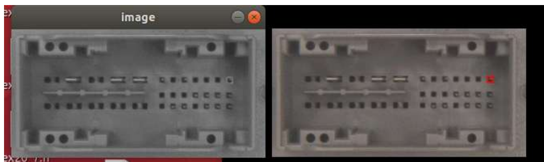
Fig. 2.2-18 OPC UA Publish-Subscribe 20 channel image transmission for ECU automatic optical inspection process in the automotive manufacturing: the received image in grayscale and the target image.
